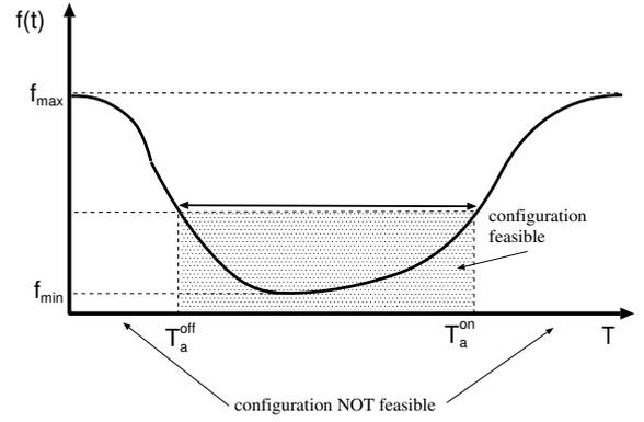
**Figure 2: Sketch of a traffic profile with indication on how to derive the switching times.**
