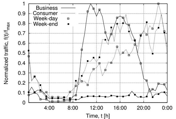
**Figure 1: Daily traffic profiles for a cell in a business area and a cell in a consumer area, week-day and week-end profiles measured in a network in operation.**
